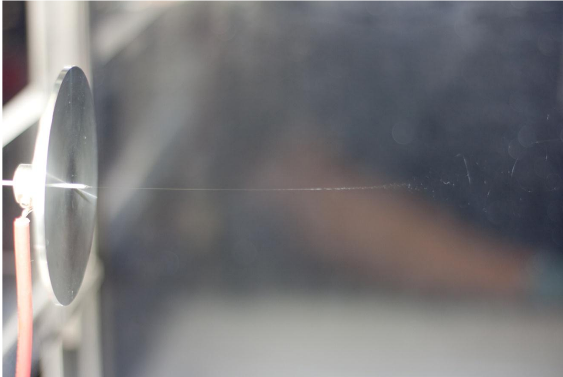
Fig. 4.7. View of needle with fiber destabilization and start of whipping motion
